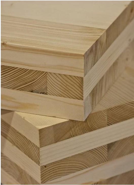
CLT Photo: https://www.usda.gov/media/blog/2018/03/30/blast-testing-shows-clt-can-take-heat
